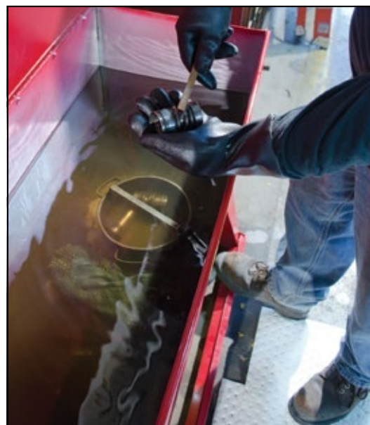
Stepping on foot treadle opens the rinse tank cover, leaving hands free for cleaning.
