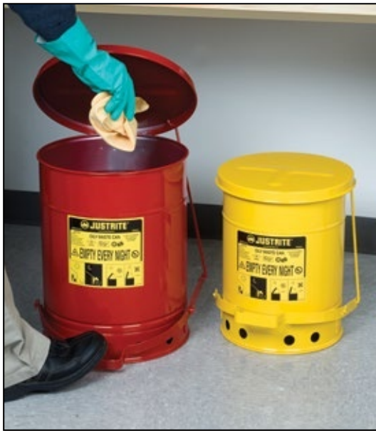
Foot pedal provides hands-free opening. When released, cover self-closes to reduce oxygen source and prevent a fire from starting.
